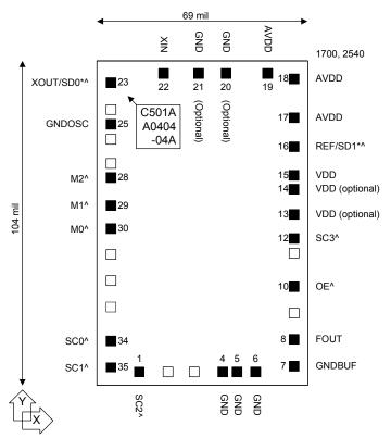
Note: ^: Internal pull-up resistor ( $120k\Omega$  for SD0,  $30~k\Omega$  for SC0-SC2, SD1, M0-M2 and OE). The internal pull-up resistor results in a default high value when no pull-down resistor is connected to this pin.
